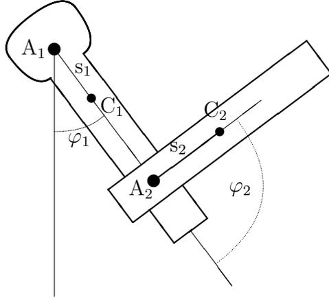
FIGURE 1. Planar double pendulum. The first pendulum swings around a fixed axis  $A_1$  and carries the axis  $A_2$  of the second body. The centers of gravity  $C_1$  and  $C_2$  are distances  $s_1$  and  $s_2$  apart from the axes; the distance between  $A_1$  and  $A_2$  is  $a$ . The configuration is determined by the two angles  $\varphi_1$  and  $\varphi_2$ .
